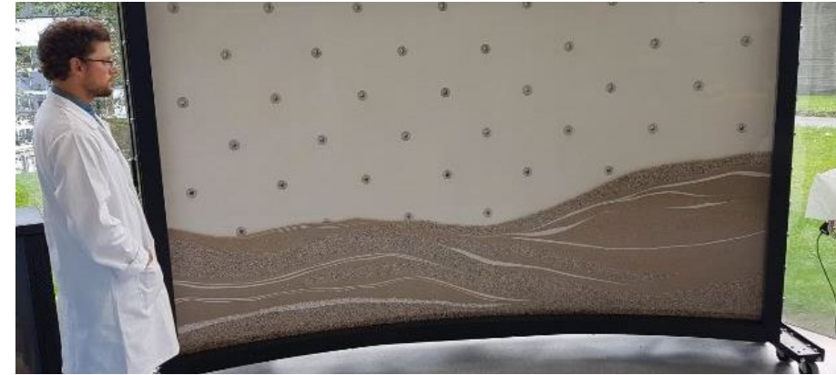
FluidFlower Rig - Intended Geometry motivated by a Norwegian reservoir
